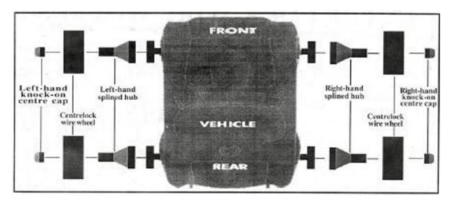
A centre-lock wire wheel is fitted onto a car axle using a splined hub: the splines (or serrations) of the hub lock with he splines on the inside of the wheel centre to produce drive. Splined hubs may be integral fitting or bolt-on. Please refer to the vehicles service manual for instructions on fitting integral splines. The diagram below illustrates fitting bolts on hubs.
